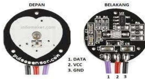
**Gambar 2.1 Sensor *Pulse***
