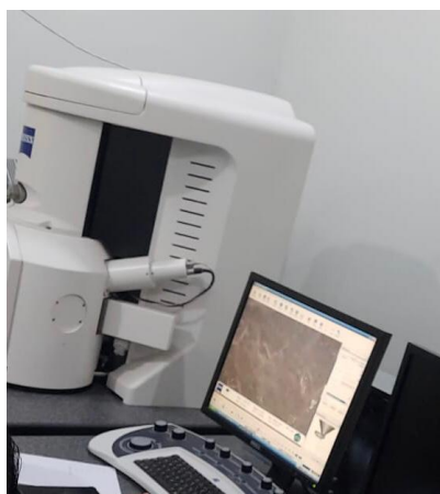
Figure 3. Scanning electron microscope test equipment
