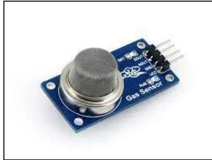
**Gambar 2.4** Sensor Asap MQ135
