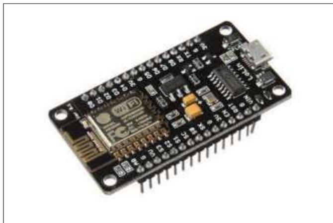
**Gambar 2.2** NodeMCU ESP8266
