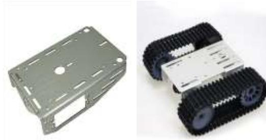
Gambar 2.10 Aluminium Chassis Frame
