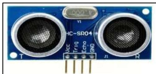
Gambar 2.14 Sensor Ultrasonik
