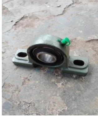
Gambar 2.8 Bearing Block (Sumber: Dokumen Pribadi)
