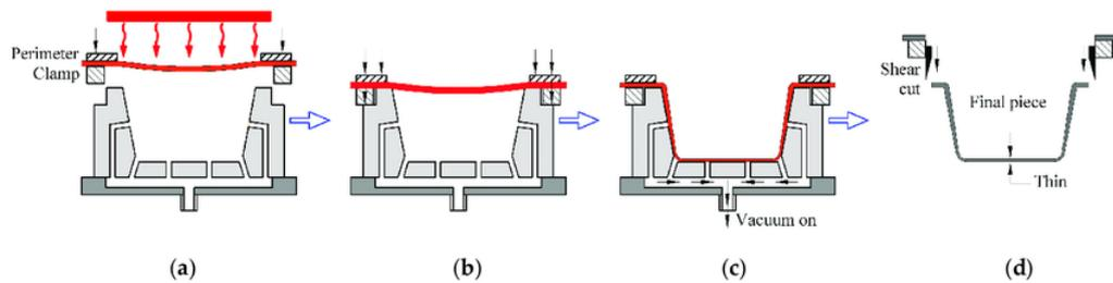
**Gambar 2.2** Proses *Vacuum forming* (Polymers, 2018)
