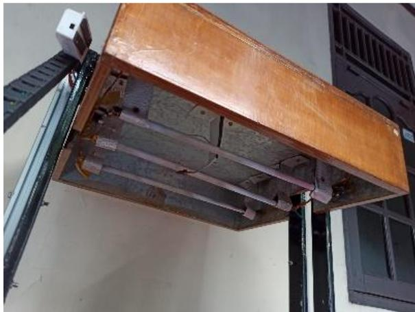
**Gambar 2.3** Kotak *Heater* (Fazlan, 2022)
