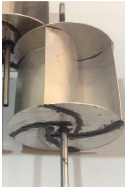
Gambar 2.1 Turbin Angin Savonius (Jamal, 2019)
