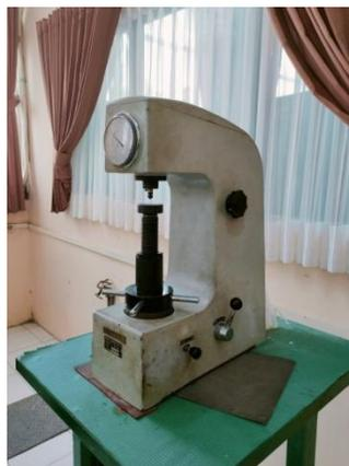
Gambar 2.3. *Rockwell Hardness Tester* Model HR-150A
