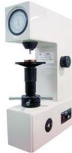
Gambar 2.4 *Rockwell Hardness Tester* (Romli, 2017)
