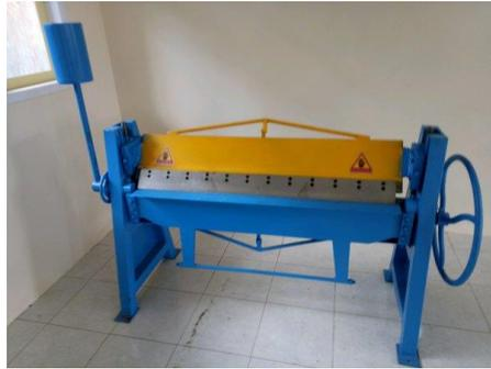
Gambar 2.23 Mesin Bending
