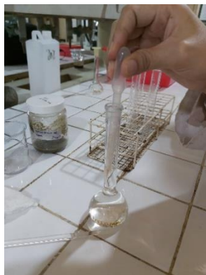
Gambar C.38 Memipet 1 ml Larutan Kasein.
