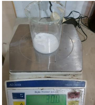
Gambar C.29 Menimbang 30 gram Amonium Sulfat.
