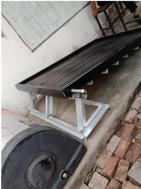
Gambar 19. Solar Water Heater Tampak samping
