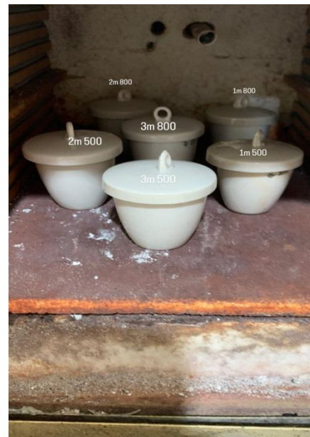
Gambar C.12 Analisa kadar mudah zat menguap
