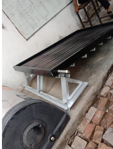
Gambar 19. Solar Water Heater Tampak Samping
