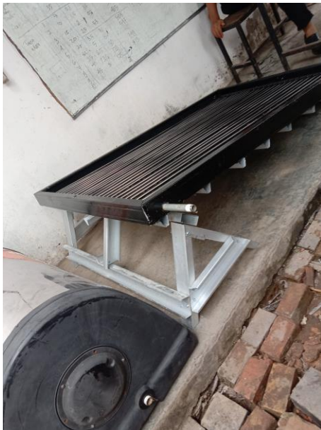
Gambar 19. Solar Water Heater Tampak samping
