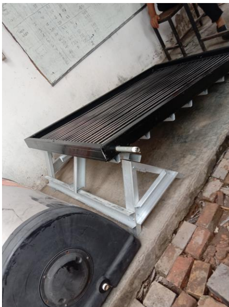
Gambar 5.19. Solar Water Heater Tampak Samping
