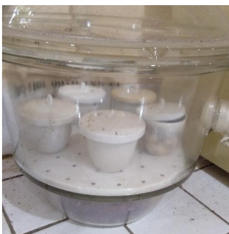
Gambar C.11. Mendinginkan didalam desikator.
