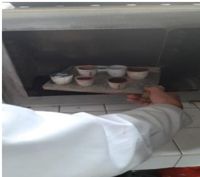
Gambar C.13. Pengujian kadar air
