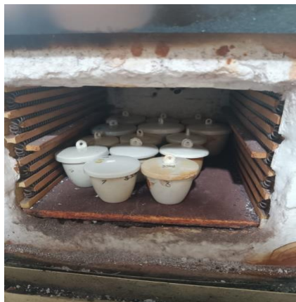
Gambar C. 15. Pengujian Kadar Volatile Matter
