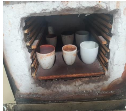
Gambar C.14. Pengujian Kadar Abu
