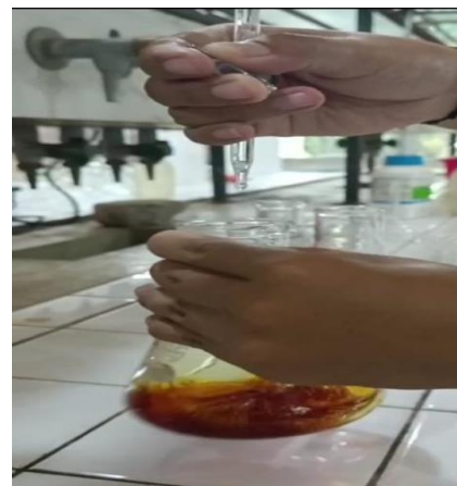
Gambar C.16. Pengujian Daya Serap Iod
