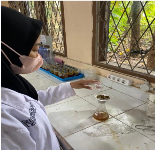
Gambar C.19. Proses pencucian daun nanas sampai pH netral
