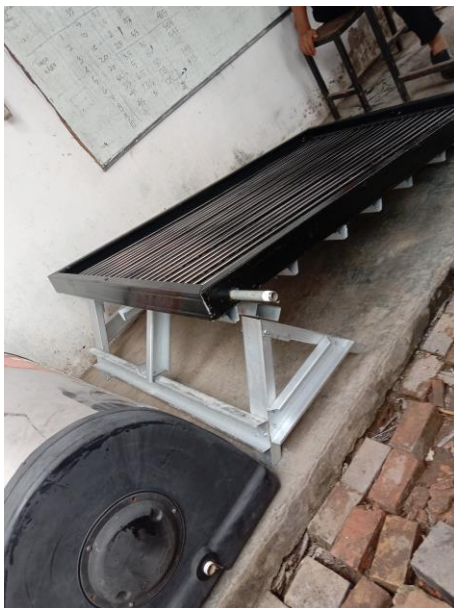
Gambar 19. Solar Water Heater Tampak samping
