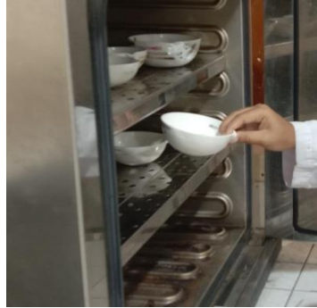
Gambar C.13 Uji Padatan Total
