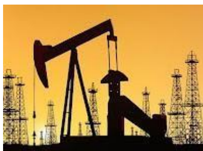
Gambar 2.6 Pumping unit ( Sucker Rod Pump )
