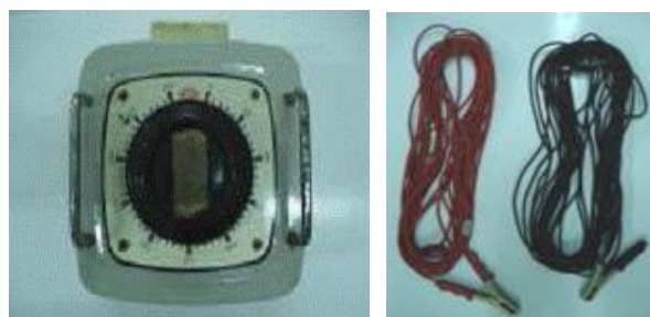
Gambar 2.19 Voltage Slide Regulator 31
