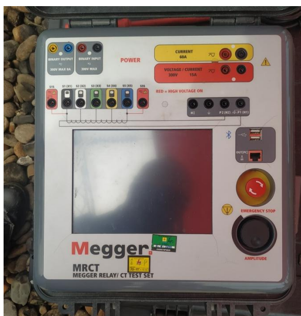
Gambar 2.14 Alat Uji Ratio Test
