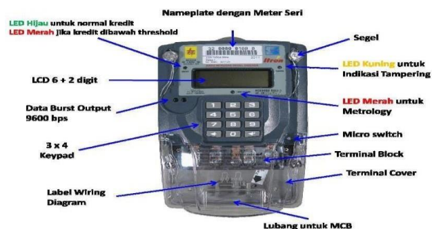
Gambar 2.14 kWh Meter Digital (Prabayar)
