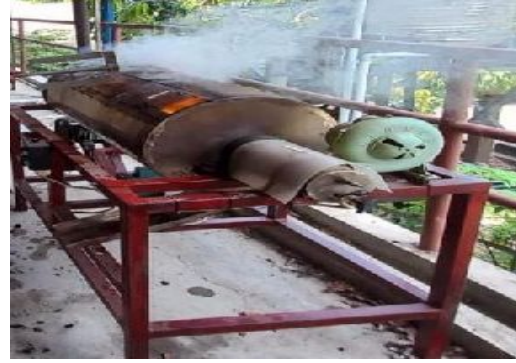
Figure 4. The Innovation Result of Rotary Furnace To Make Shell Charcoal Into Briquette
