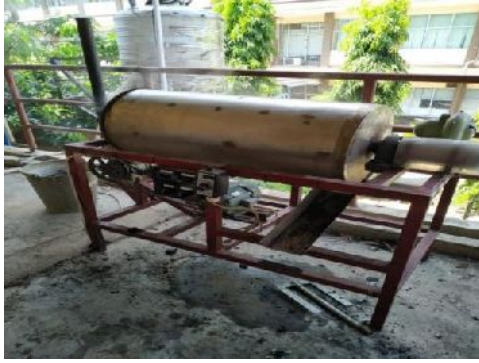
Figure 2 The Innovation Technology of Rotary Furnac for Making charcoal from coconut Shell was Studied
