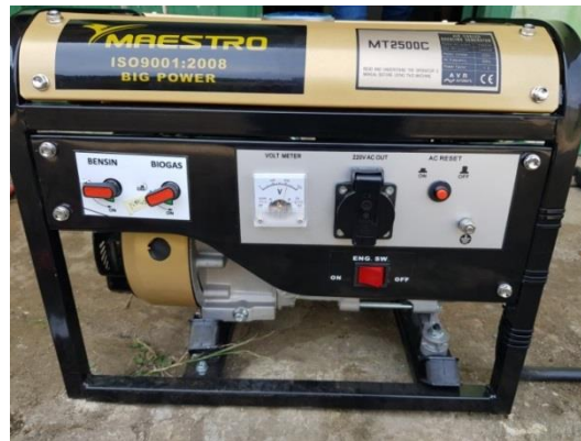
Fig 1. Modified Generator Set
