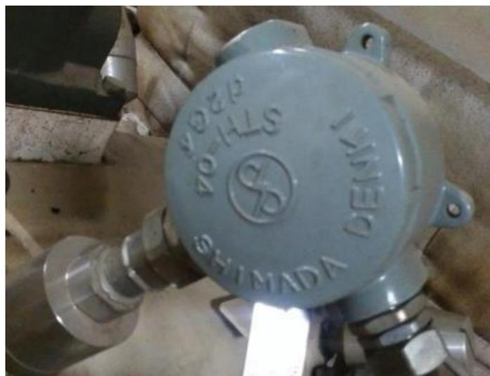
**Gambar 2.11** Relay *Overspeed*
