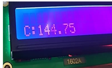
Gambar 11. Suhu Medium Roasting 15 Kg
