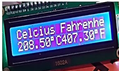
Gambar 16. Suhu Dark Roasting 20 Kg
