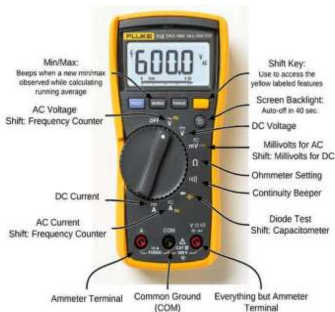
Gambar 2.17 Multimeter Digital
