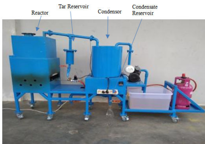
Figure 1. LDPE pyrolysis equipment
