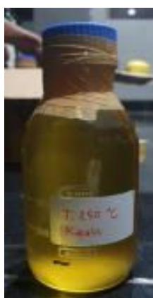
Figure 2. Fuel converted from LDPE plastic waste
