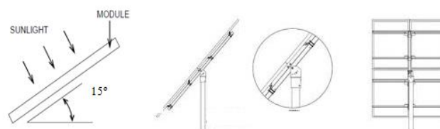
Fig 4. Design of fixed panel system
