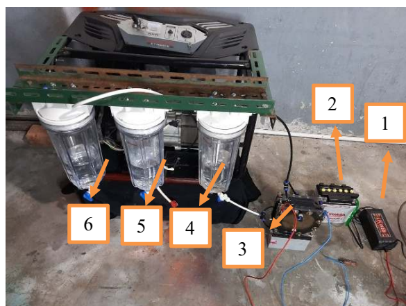
Figure 7. HHO Generator Installation
