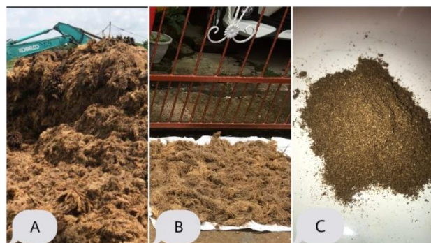
Figure 1. Preparation of Palm Oil Bunches (A) Palm Oil Bunch Waste, (B) Palm Oil Bunches, (C) Small Size Palm Oil Bunch
