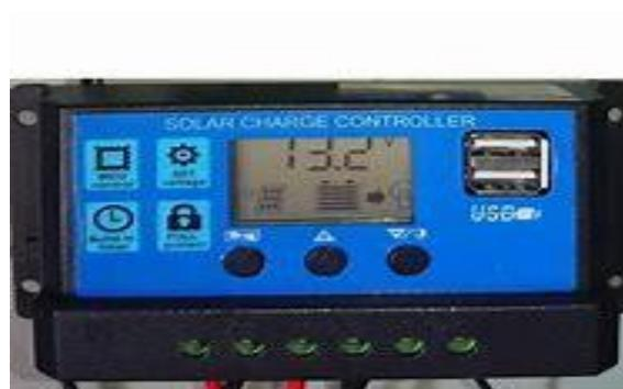
**Gambar 2.8** Solar Charge Controller (SCC)
