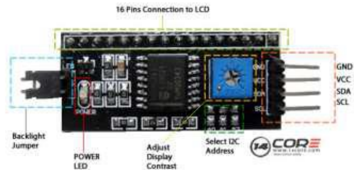
Gambar 2.13 Susunan Pin Out I2C Serial Interface [11]
