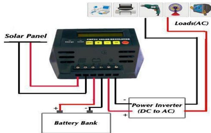
Gambar 2.11 Prinsip Kerja Solar Charger Controller
