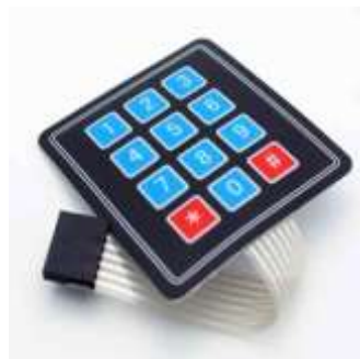
Gambar 2. 10 Keypad Matrix 4x3
