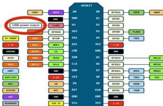
Gambar 2.9 GPIO NodeMCU ESP8266 v3 <sup>[4]</sup>
