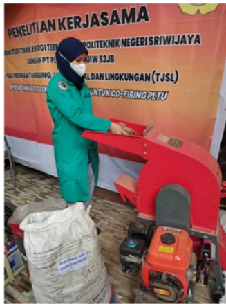
Fig. 3. EFB Size Reduction
