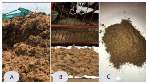
Figure 1. Preparation of Palm Oil Bunches (A) Palm Oil Bunch Waste, (B) Palm Oil Bunches, (C) Small Size Palm Oil Bunch
