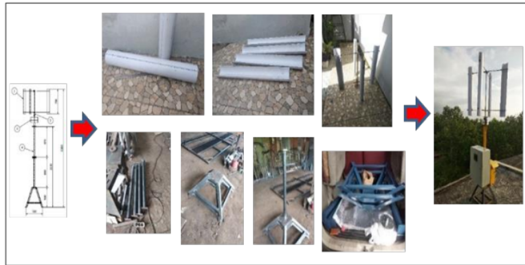
Figure 4. Fabrication Process of Giromill Wind Turbine
