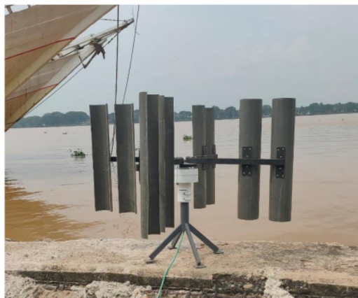
Figure 3. Darrieus H Blade Model
