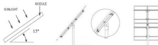
Fig 4. Design of fixed panel system
