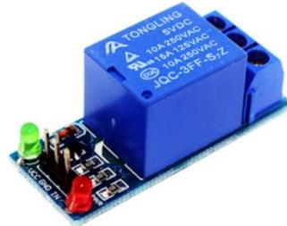
**Gambar 2. 9** Modul relay 5 Volt
