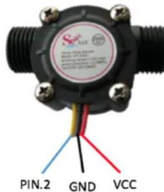
**Gambar 2. 6** *Water flow sensor*
