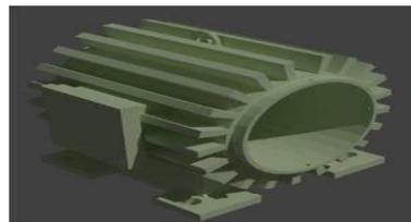
**Gambar 2.3** Frame Stator
