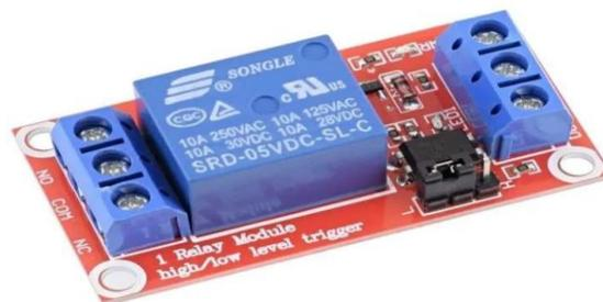
**Gambar 2.4** Modul Relay<sup>[6]</sup>
