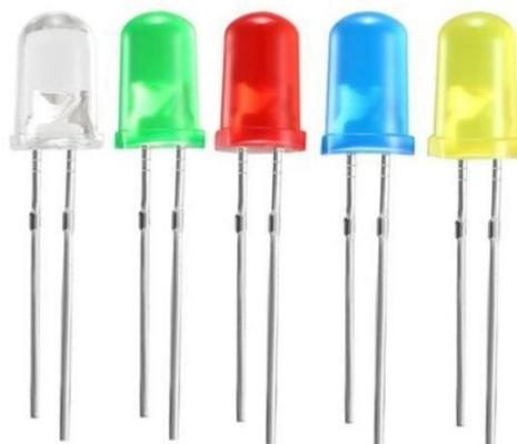
Gambar 2.10 *Light Emitting Diode (LED)*<sup>[12]</sup>
