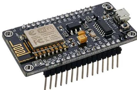
**Gambar 2.2** NodeMCU ESP8266
