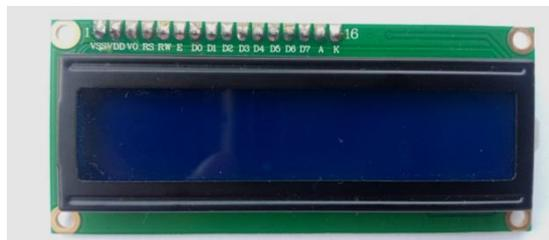
**Gambar 2.7** LCD (*Liquid Crystal Display*) 16 x 2
