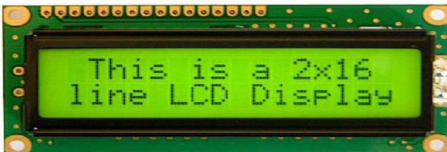
**Gambar 2.18** LCD 16 x 2
