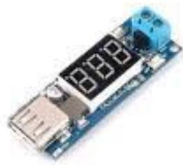
**Gambar 2.17** DC to DC Converter LM2596
